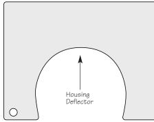
deflector will redirect the camera's flash to the EV Controller which controls the external strobe output. To attach, push the deflector over the back of the housing port until the deflector clips into position, blocking the camera flash.
